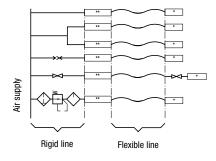
The air fuse should be installed directly between fixed or rigid pipework and the flexible tube to protect the whole length of the flexible tube. Only tubing **after** the air fuse is protected. The air fuse must be installed in the correct orientation. Failure to do this will render it ineffective. When a shut off valve is located before the air fuse, the valve must be opened slowly in order to control initial air flow and avoid decompression effects which may trip the air fuse.
